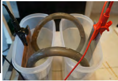
Bridge 1 inch brine filled open ended polythene tubing.
